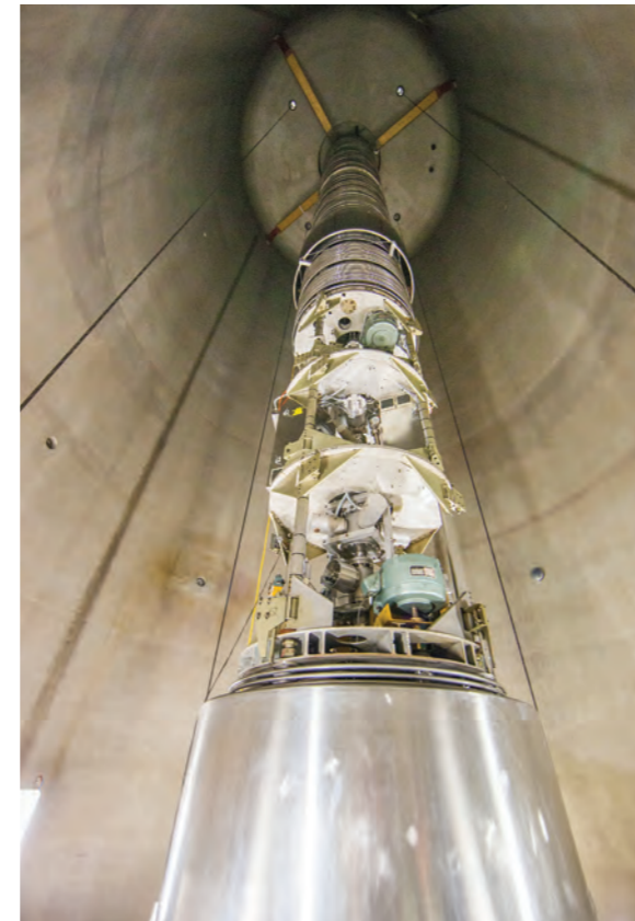
The high voltage terminal at the heart of the 14UD Pelletron Heavy Ion Accelerator, providing accelerated ion beams at HIAF
