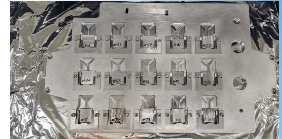
Aluminium matrix metal composites (MMCs) samples mounted in the HIAF-SIBL materials test frame.
