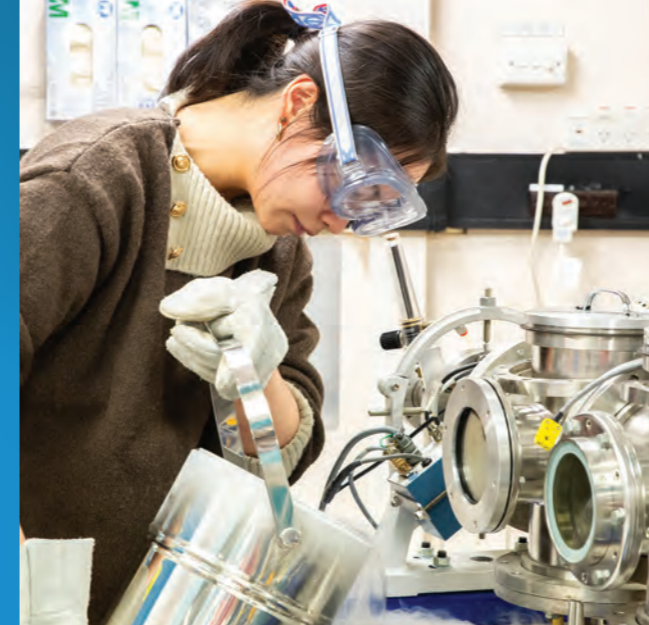
Using liquid nitrogen: the iLab implanter’s flexible capabilities include heating and cooling samples across a wide range of temperatures.
